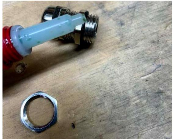
16. Remove 5" of the new grounded cord sheathing and add the cable gland nut
