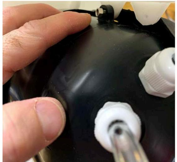
30. Insert backplate on to the tank and tighten all 4 screws. Be careful not to over-tighten
