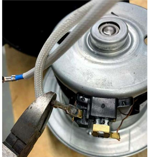
14. Use rotary tool or any kind of cutting tool to remove soldered on quick disconnect from the motor terminal without removing terminal
