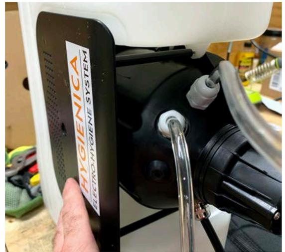
31. Insert hoses back into the tank and use WD40 on both hose connections. This will help getting them back in and making an air tight connection
