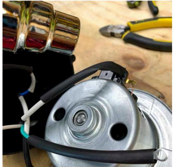
24. Use a heat gun to shrink the tubing on to the green wire for a tight fit and use a M4-0.7 6mm pan head screw to attach ground wire to motor housing.
