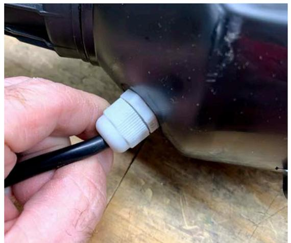
10. Remove heat shrink tubing from the brown wire of the power cord (keep the heat shrink tubing on the brown wire from the switch)
