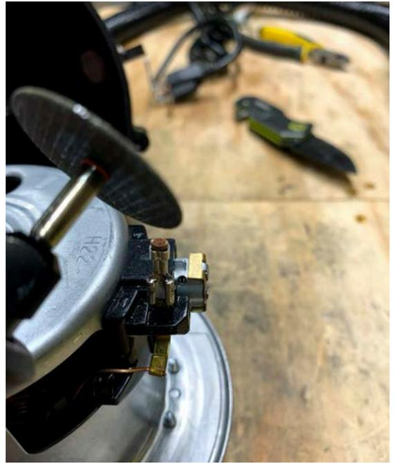
15. Remove power cord and nylon cable gland from motor housing and add brass cable gland with LOCTITE to motor housing
