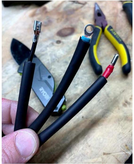
21. Put both end of the bullet connections together, cover with heat shrink tubing then use heat gun to properly shrink tubing for tight fit
