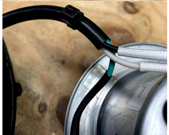
26. Put the gasket back on the motor and insert back into the motor housing. Be sure to pull the power cord out slowly through the cable gland until the zip tie reaches the cable gland.
