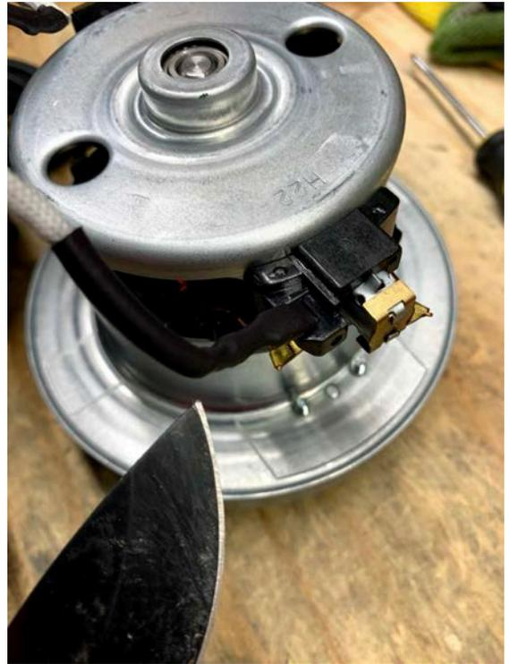
11. Remove heat shrink tubing on the blue 2 wires
