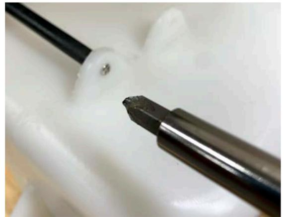
6. Remove the 5 screws that hold the motor guard on the motor housing and remove guard
