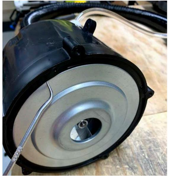
8. Use needle nose pliers to pull the gasket completely out
