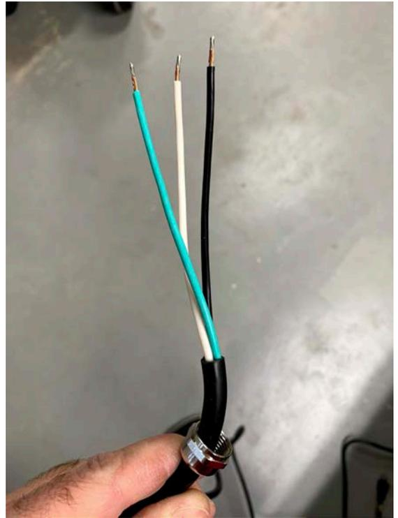
17. Insert power cord in to the motor housing
