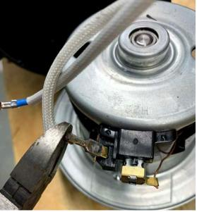
14. Use rotary tool or any kind of cutting tool to remove soldered on quick disconnect from the motor terminal without removing terminal
