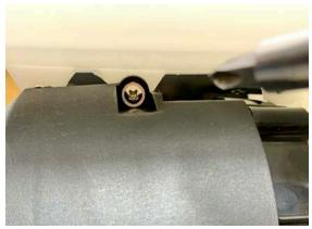
4. Make sure to remove the nuts from the motor housing
