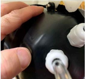
30.Insert backplate on to the tank and tighten all 4 screws. Be careful not to over-tighten
