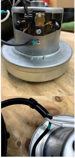
26. Put the gasket back on the motor and insert back into the motor housing. Be sure to pull the power cord out slowly through the cable gland until the zip tie reaches the cable gland.
