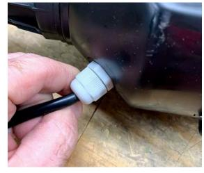
10. Remove heat shrink tubing from the brown wire of the power cord (keep the heat shrink tubing on the brown wire from the switch)
